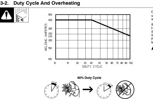
Duty Cycle is percentage of 10 minutes that unit can weld at rated load without overheating.
